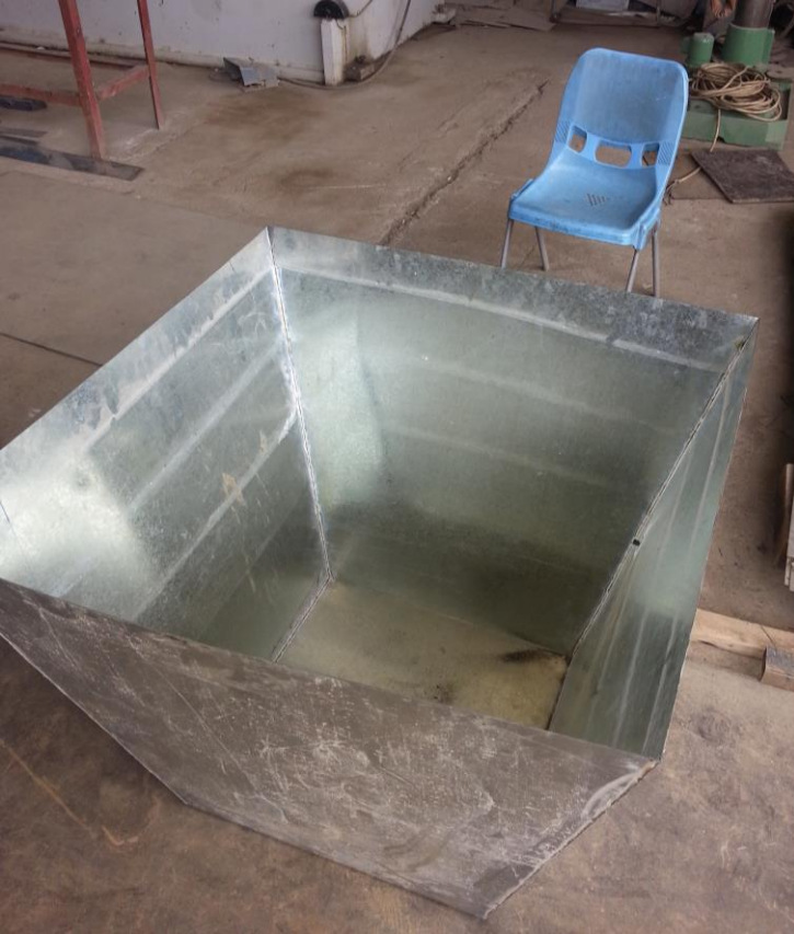
Solar pond (Trapezoidal shape) manufacturing Base dimensions = 60×60 cm Top surface dimensions = 92×92 cm Height = 86 cm obliqueness angle ( \theta ) = 12°
