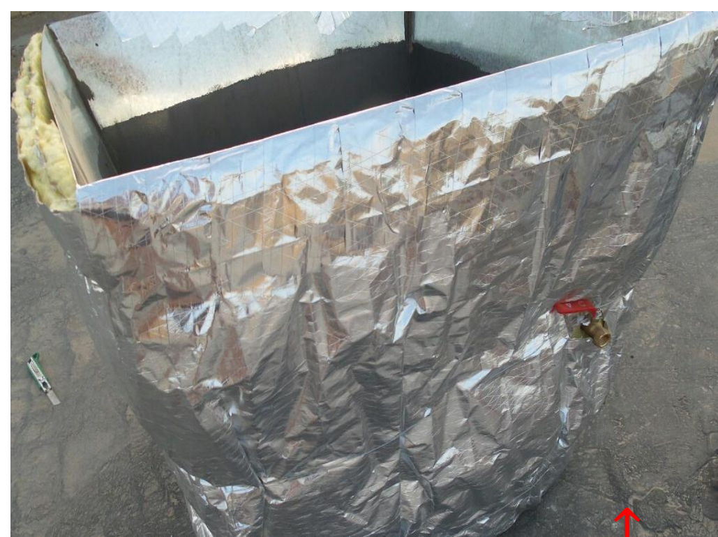
Coal tar Epoxy lining and double layers of Isolation glass wool (5 cm thick)
