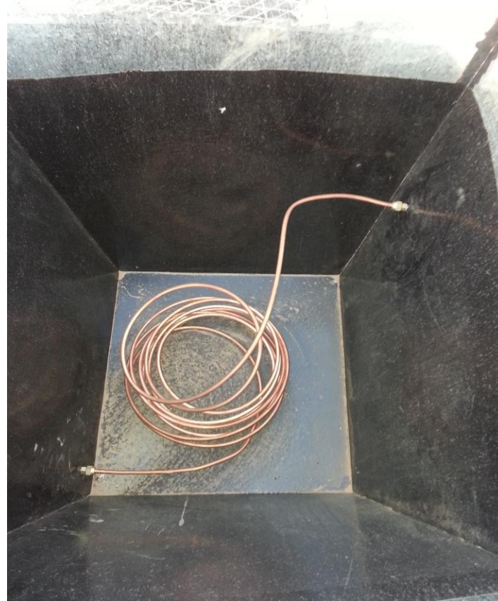
Internal coil exchanger fixed inside solar pond at lower layer (heat store layer) Diameter = 3/8 inch Length = 10 m
